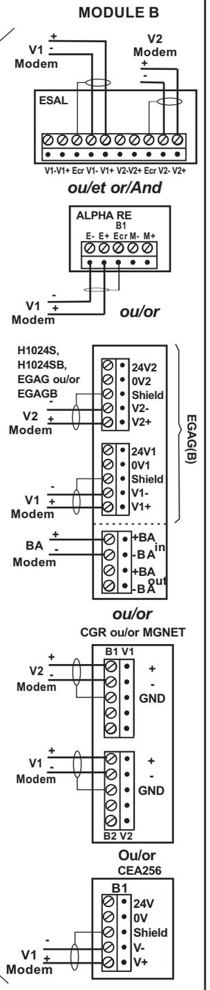
The communication links are wired with duplex cable 8/10th SYT1
