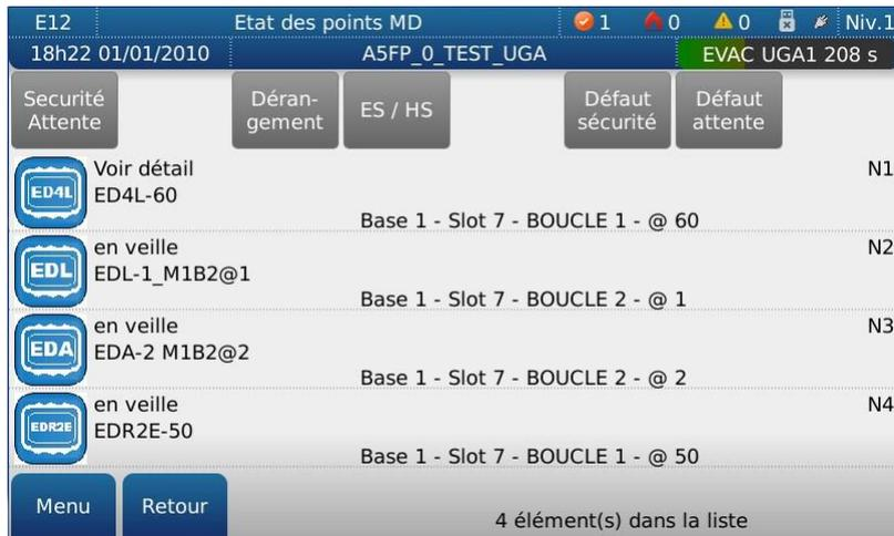
The screenshot displays a software interface for fire alarm management. At the top, it shows 'E12', 'Etat des points MD', and 'Niv.1'. The time is '18h22 01/01/2010' and the location is 'A5FP\_0\_TEST\_UGA'. A green bar indicates 'EVAC UGA1 208 s'. Below this are several control buttons: 'Sécurité Attente', 'Dérangement', 'ES / HS', 'Défaut sécurité', and 'Défaut attente'. The main area contains a list of points with their status and location:
